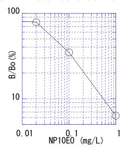
This test kit has a wide detection range between 0.02mg/ and 1mg/L.
